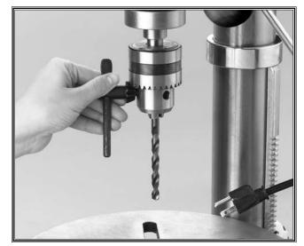
Figure 33. Chuck key engaged.
